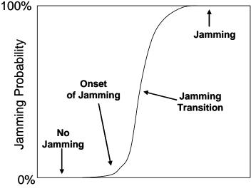
Particle Diameter / Orifice Diameter
